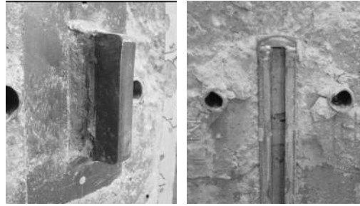
Figure 7. Shear bracket and inverted U-shaped steel box after testing
